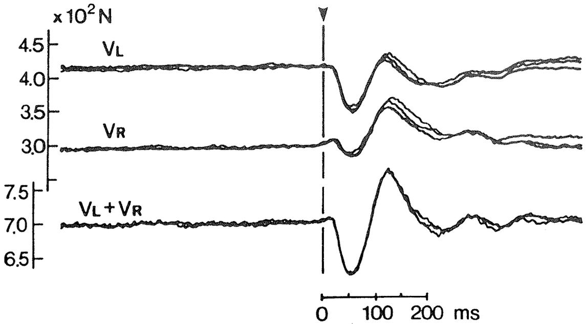
Fig. 1. The vertical reaction forces at the releasing movement ( $\blacktriangledown$ ) in the world-class archer (overlapped in 3 trials). Upper three traces show the total forces in left foot. Middle three traces show the total forces in right foot. Lower three traces show the total forces in both feet.
